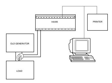
The RS232 cable uses the upper terminal bracket on the back of the Hawk. The cable (not supplied) is connected to your printer, which is programmed to print out the following line when a change in the alarm status occurs: TYPE, PV, AL1, AL2, STA.
