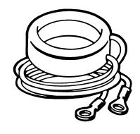
Donut Current Transformers enable the Hawk to monitor AC current up to 1,999 (HK 35) amps or 19,999 (HK 45) amps. The Donut (also known as a "Toroid") is placed around one of the legs of the device being monitored, and emits up to a 5 amp signal. The HAWK can be scaled to accurately display the current being monitored. Each Donut comes with 2' long secondary leads.
