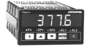
By using the password feature, the meter's programming functions and set points are protected from accidental reprogramming.
